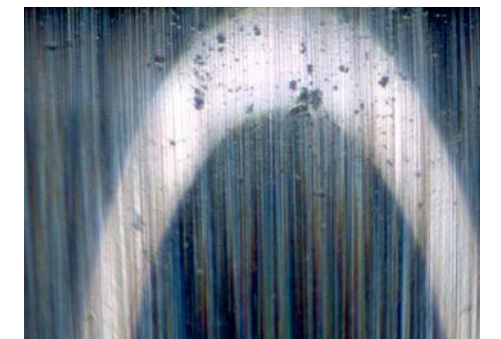
Indentations in raceway caused by particles
